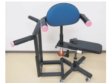
Nursing care device (lifter and mover) developed by high school students 高校生が開発した介護用機器（移乗機）
