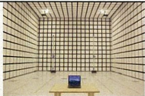
(10m法電波暗室)
