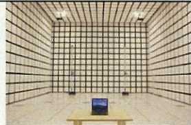
(10m法電波暗室)
